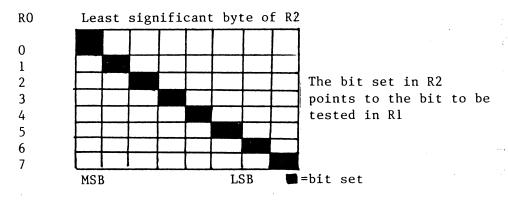
COC R2,R1 (Compare Ones Corresponding), sees whether the bits set in R2 are also set in R1; if so, then the equal flag ST2 is set. The JNE (Jump Not Equal) operates if the relevant screen bit was not set. Using this, the status of a screen bit can be tested and acted upon.
